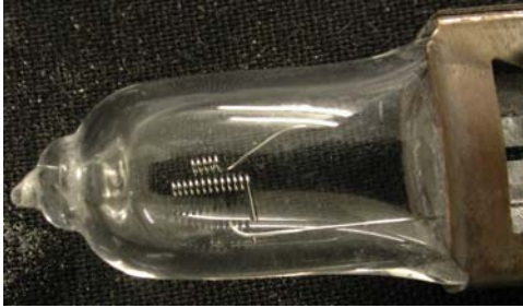
Cold fracture of a filament coil.
