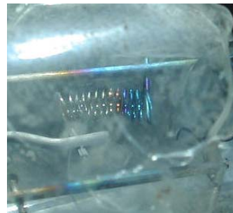
Filament heated by neighbouring coil. Note the tinting.
