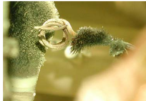
Heavy oxidation caused by exposure to air whilst incandescent
