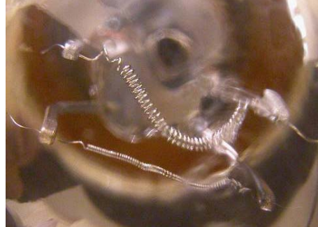
Dual filament brake/tail lamp. The finer tail filament was not incandescent, but was heated by the lit brake coil.
